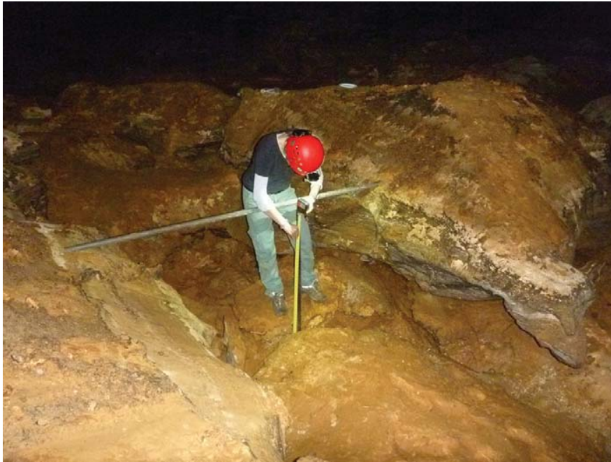
Figure 16: Using a tape measure and steel ruler to measure groundwater depth in Flat Roof 1, Jewel Cave, July 2012. Photo by Stefan Eberhard.
