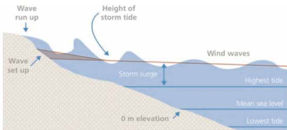
Figure 16: Storm surge temporarily increases sea levels during severe weather events
